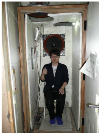
Figure 4: Low Frequency Sound Chamber and Subject
